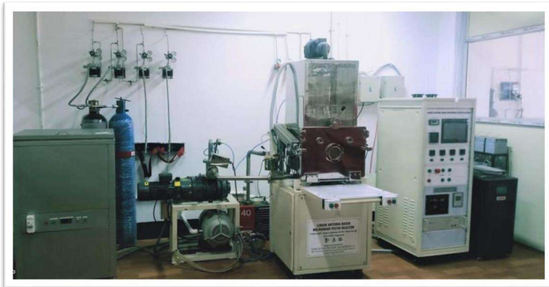
Fig.1: Fabricated linear antenna based MWPECVD unit (Made in India) of 2.45 GHz frequency and installed at Meghnad Saha Institute of Technology .
