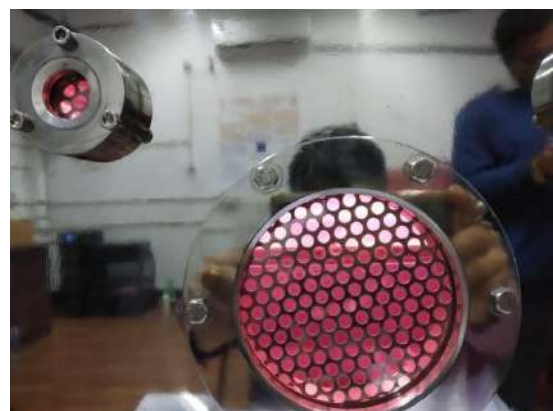
Fig2- Appearance of DLN coating by MWPECVD Fig3.- Uniform plasma glow as seen from chamber window.
